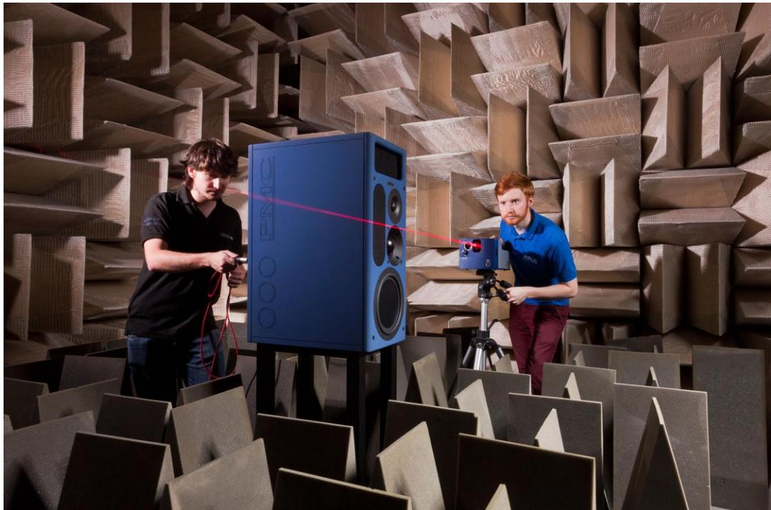
Oliver Thomas (left) in the NPL 'Hemi' anechoic chamber, the latter augmented by a scattering of floor wedges.
