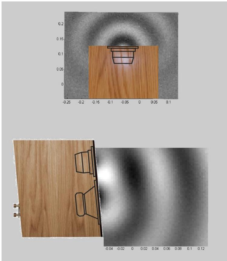
Here is a top view and side view of the wave propagated output, near crossover of a two way 'fact' loudspeaker
