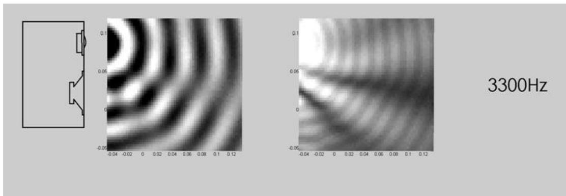
A trial two way system with a passive second order crossover showing some interference between the driver outputs, ie not ideally integrated
