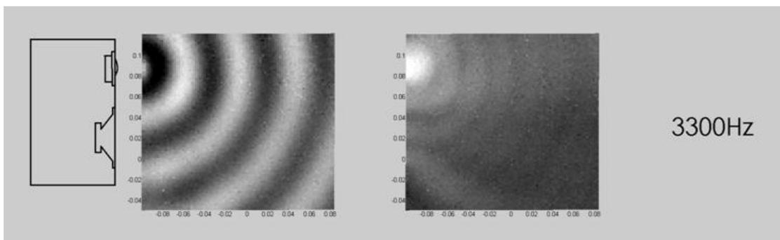
The same system but in active form proving tighter driver control plus a steeper rolloff fourth order filter. The same crossover frequency now shows improved radiated wave coherence.
