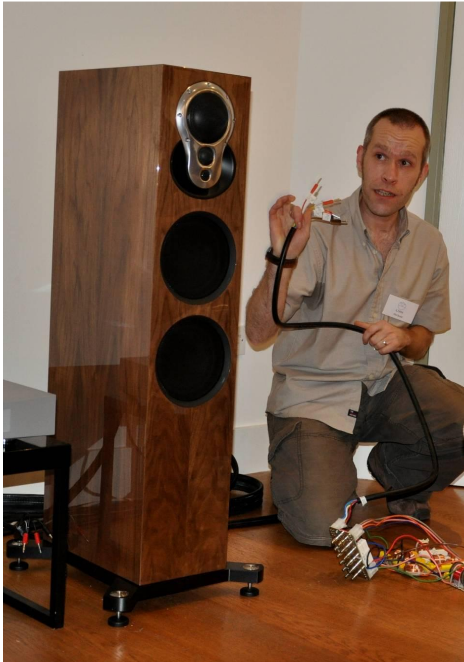
Phil Budd – Senior Acoustic Engineer discussing active-v-passive operation for the Akurate 242, '5' way loudspeaker, in gloss finish. The photo by chance brings out the multi-way connector panel (the silver connector board) for the crossover which allows for single and multi -way wiring and then for direct connection for active operation in conjunction with an external line level active filter crossover
