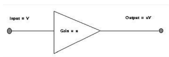
Fig.1 In an amplifier without feedback, the output consists of the input signal multiplied by the gain  $\mu$ .
