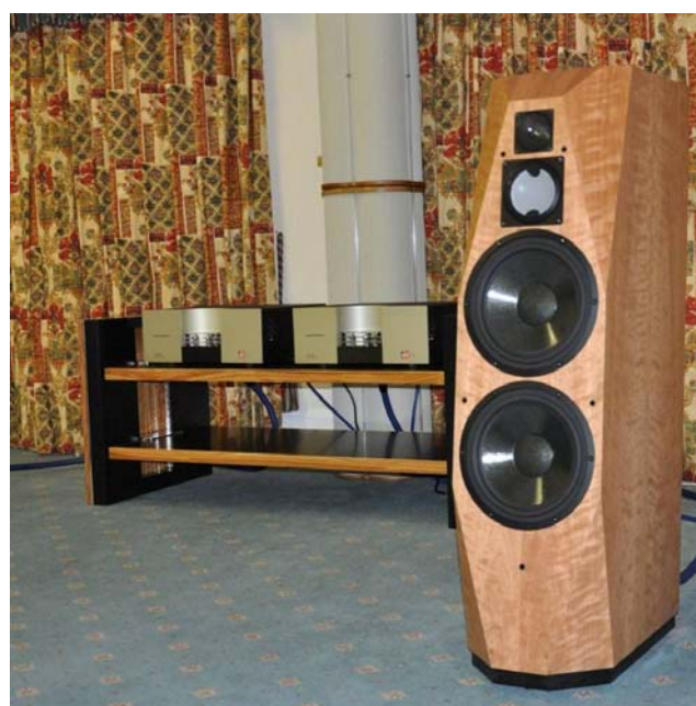
The Avalon 'Time', grille off (not for listening), bass by Eton, mid and treble by Accuton) flanked by cj LP275M all valve power amps
